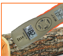
Wood moisture content measurement
