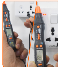
SPT Single Probe Test AC Voltage
