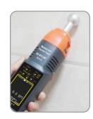
Through 'Relative Penetrate Trace' 'RPT' mode, locate the highest moisture content under the tile / Marble (MS-WITC3MT model only)
