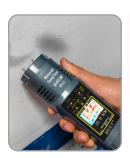
Pin type sensor measure surface moisture content
