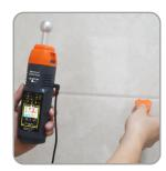
Through remote pin sensor locate moisture where hard to reach area
