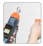
Through 'Relative Surface Trace' 'RST' mode. locate the highest moisture content on concrete
