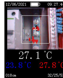
Precisely find heat map in a circuit, such as in Link / Busbar connection
