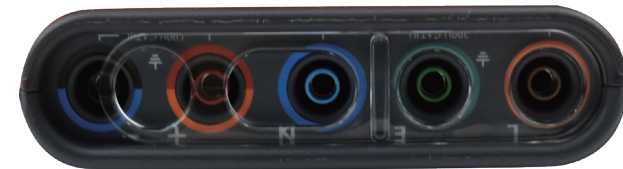
Fig.2 Interlock in position for RCD & Loop testing
