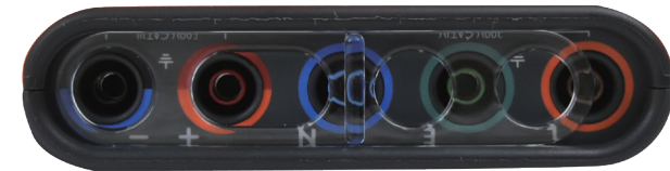
Fig.1 Interlock in position for Continuity and Insulation testing
