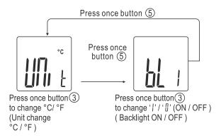
Press button (5) and hold for 3 secs. to exit setting mode.
