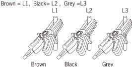
Clip on the conductor properly as shown below
