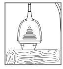
Remote pin type sense, moisture '% WME' reading
