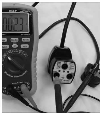
Continuity / Wiring Check
